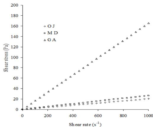
Figure 1. Rheogram of reconstituted beetroot juice for different carrier materials with original juice at constant temperature of 25°C and at constant solid content of 40%
